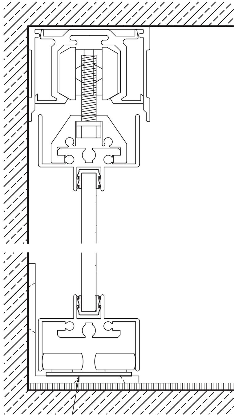
Wall connector for groundplate with rollers
