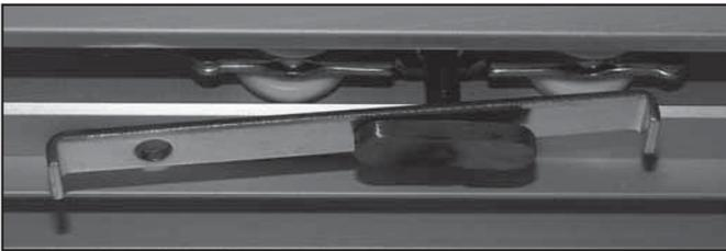
Push the top roller into the insert profile (slide rail), so that it hangs rather loosely. **Please note:** The brake must be pushed between both top rollers of the element inside the guiding track (see the picture below).
