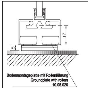
Mount the ground plate on the floor where the moving door will be situated. Use the wall outlet. For this put the door into position and mark the floor with tape where the ground plate should be positioned. If there are differences in height on the floor put a spacer between the floor and the ground plate.
